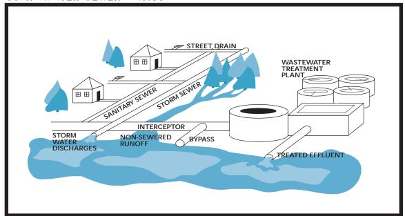
Stormwater flows into the stormwater system through a storm drain. These are frequently located along the curbs of parking lots and roadways. The grate that prevents larger objects from flowing into the storm sewer system is called a catch basin. Once below ground, the stormwater flows through pipes which lead to an outfall where the stormwater enters a stream, river or lake. In most areas of New Jersey, the stormwater sewer goes directly to local waterway without any treatment.
